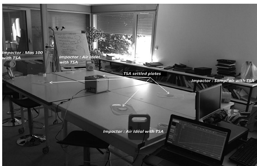
Figure 1. Layout of the different items of measurement equipment: in the center the CLEAPART-100, four culture plates 50 cm away, then four biocollectors 1 m away.
